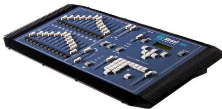
**Submaster Playbacks:** To make life a little easier on the operator these desks allow you to setup a full scene similarly to the two scene preset desk, however, the scene can then be recorded to one single fader.
