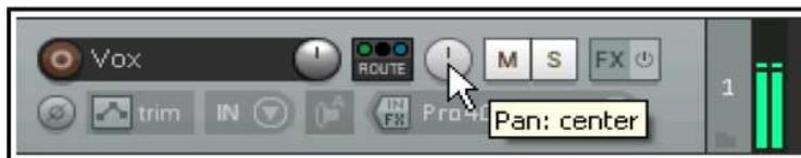
**Volume:** The rotary fader shown here is used to adjust a track's **volume**. With some layouts, this will be shown as a horizontal fader.
