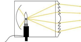
Figure 6 - Diagram showing beam in a Fresnel lantern (narrow focus)
