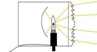
Figure 7 - Diagram showing beam in a Fresnel lantern (wide focus)
