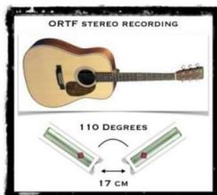
**Mics used:** Two directional mics, usually small diaphragm condensers
