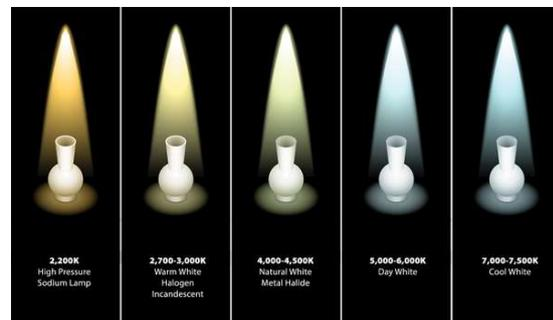
Note that the cooler the light, the higher the number. The warmer the light, the lower the number.
